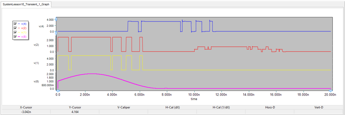
Three separate plots for v(1) , v(2) and v(4) with a time-limited sinusoidal input signal.
